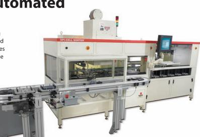
Sorts PV cells according to electrical performance
