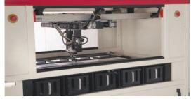
Tested cells are sorted into output bins according to the cell's electrical performance.
