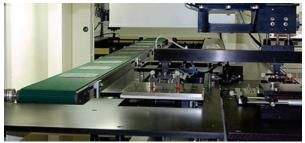
Automated cell handling gently positions each cell for electrical testing under simulated sunlight
